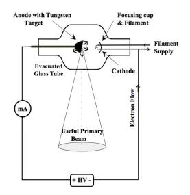
Intensity of the X-ray beam is defined as the **total energy emitted per second per unit area passing through a surface (at right angles).**
