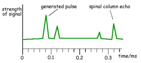
The ultrasound transducer sends **pulses** into the patient and detects the reflections from various boundaries within an organ.
